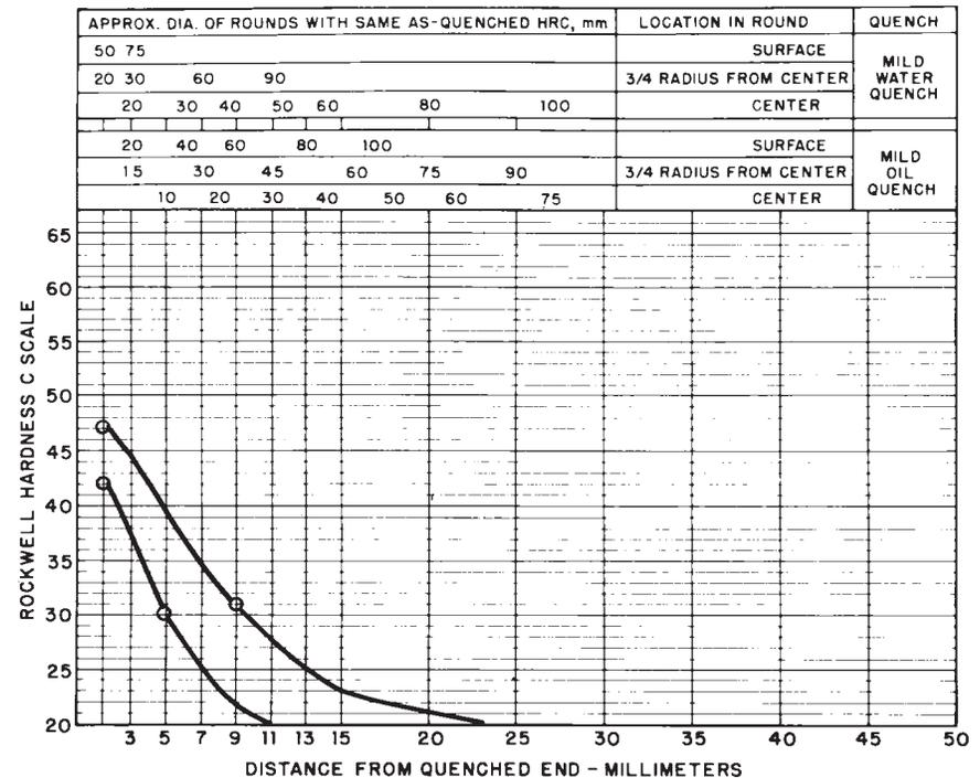
FIG. 13 Limits for Hardenability Band 4620 RH
