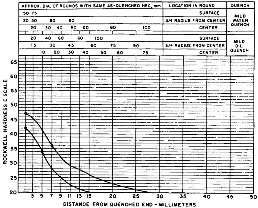
FIG. 19 Limits for Hardenability Band 8620 RH
