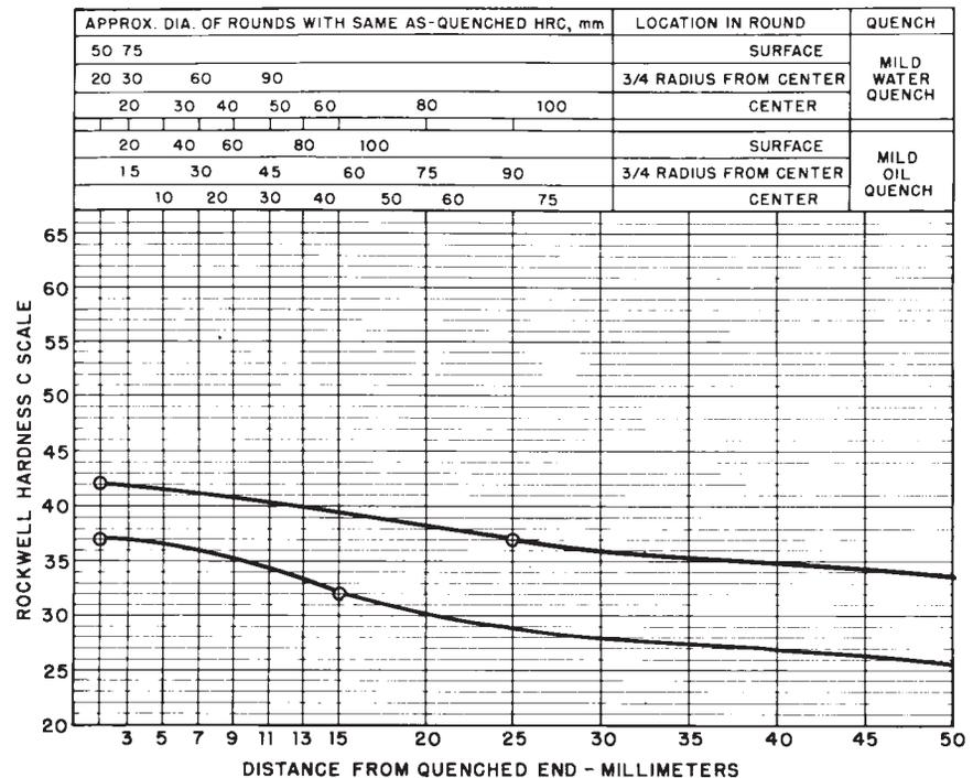
FIG. 4 Limits for Hardenability Band 3310 RH
