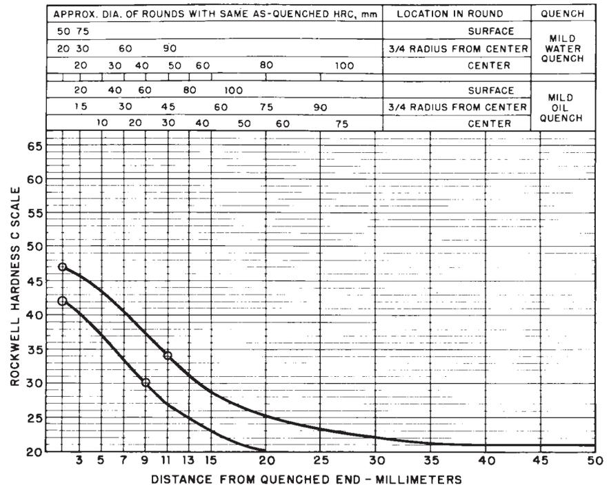
FIG. 12 Limits for Hardenability Band 4320 RH
