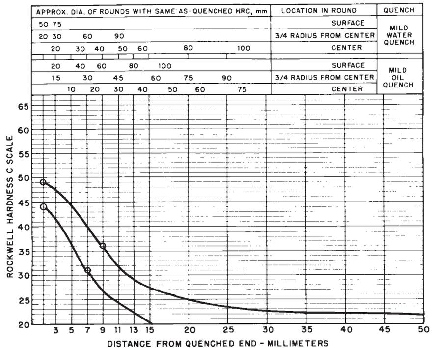
FIG. 20 Limits for Hardenability Band 8622 RH
