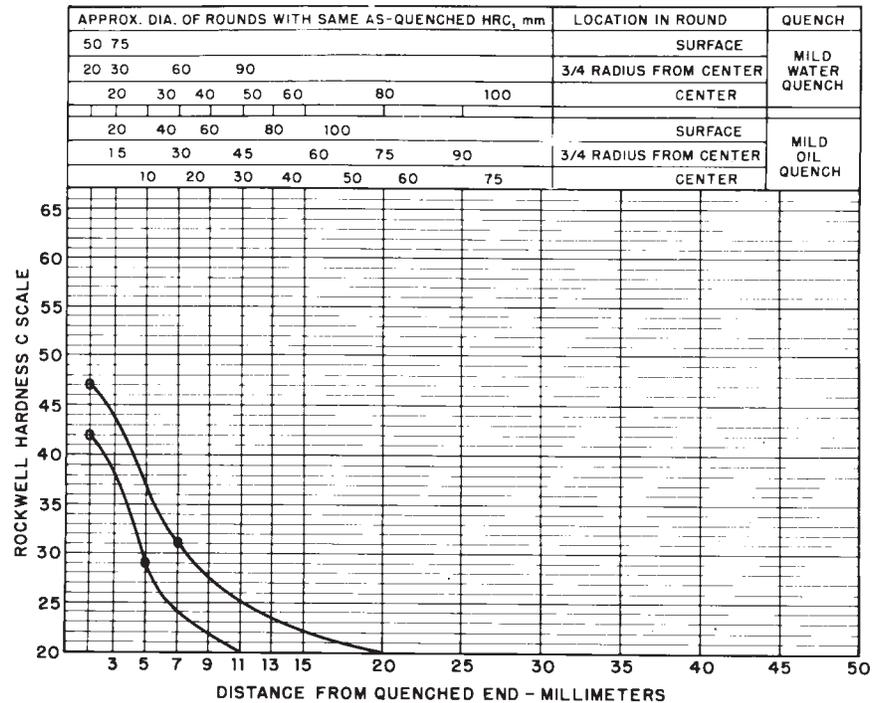
FIG. 6 Limits for Hardenability Band 4118 RH
