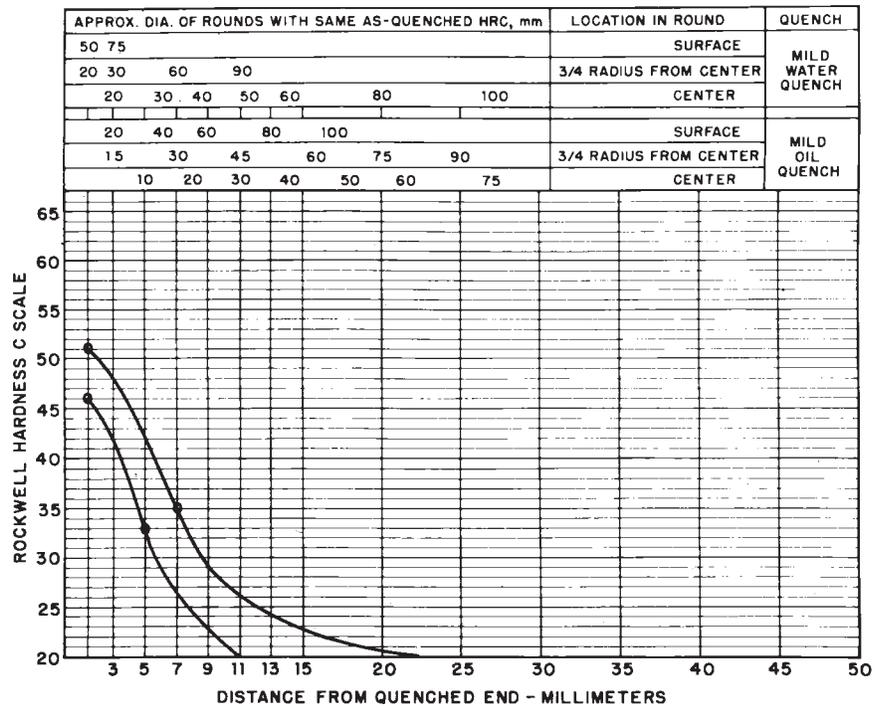
FIG. 5 Limits for Hardenability Band 4027 RH
