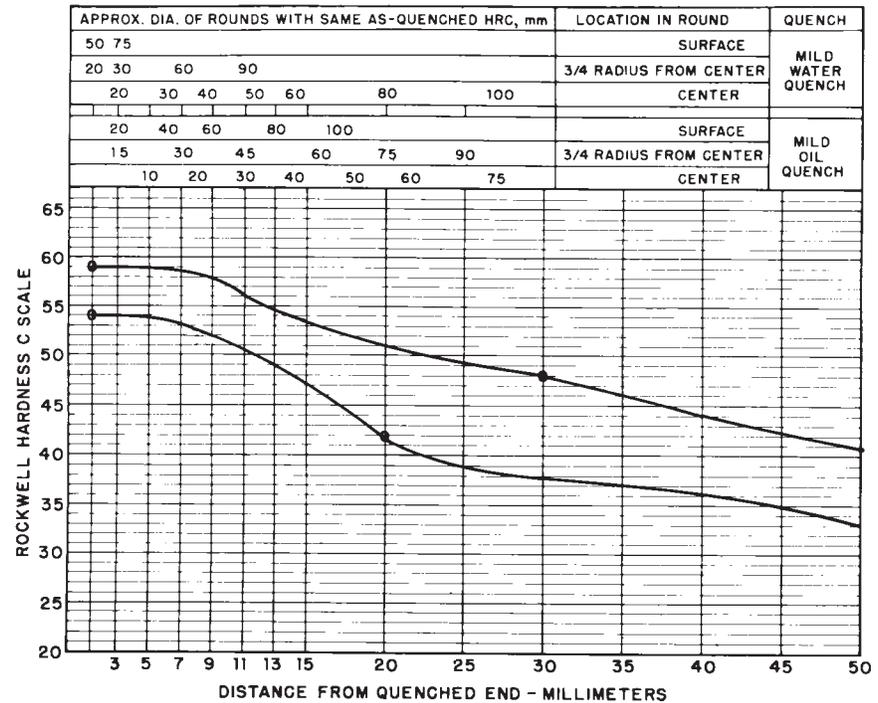
FIG. 9 Limits for Hardenability Band 4140 RH
