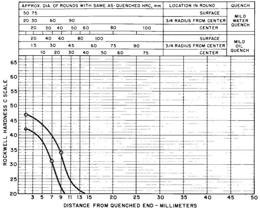
FIG. 2 Limits for Hardenability Band 15B21 RH
