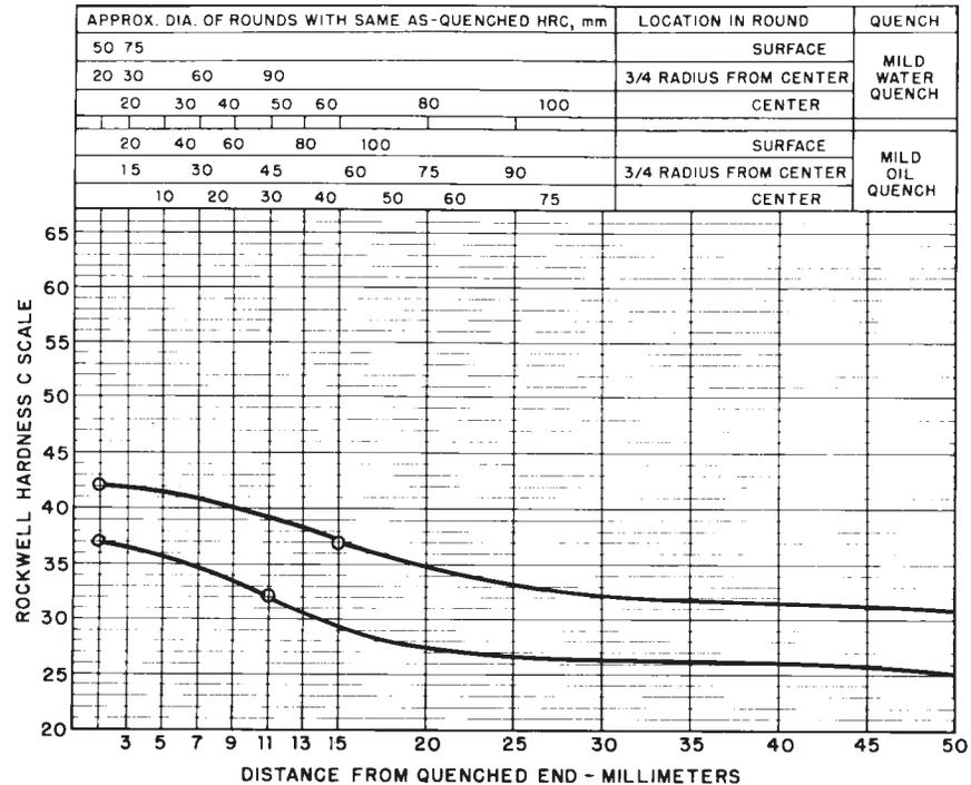
FIG. 23 Limits for Hardenability Band 9310 RH
