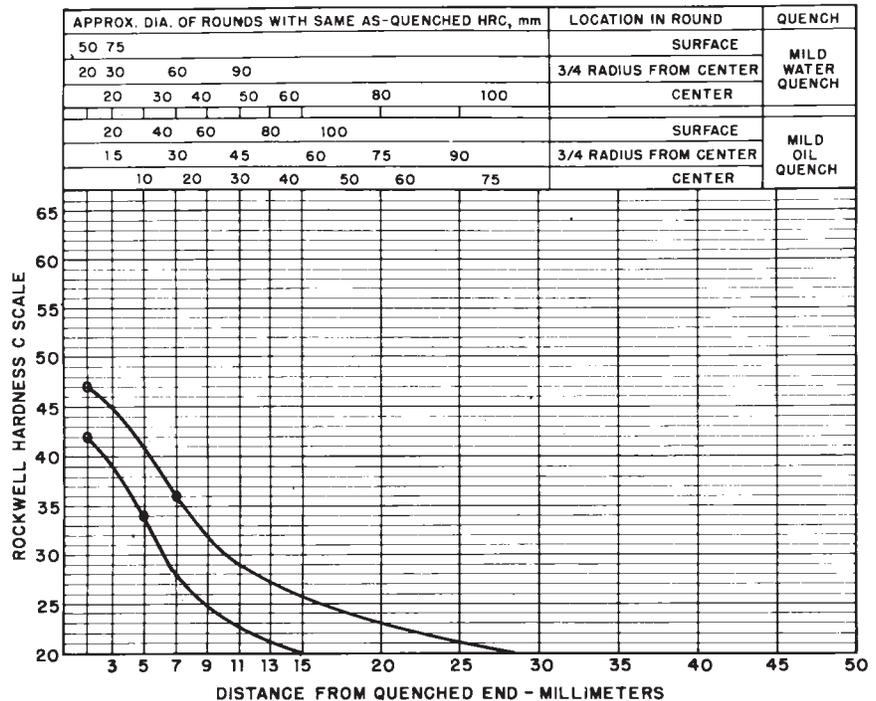
FIG. 7 Limits for Hardenability Band 4120 RH
