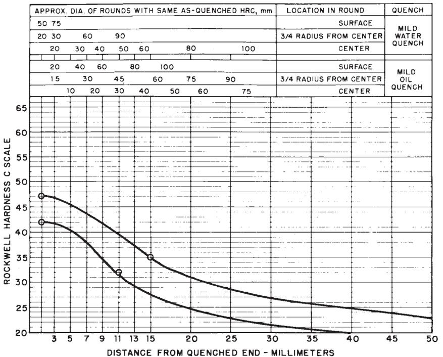
FIG. 14 Limits for Hardenability Band 4820 RH
