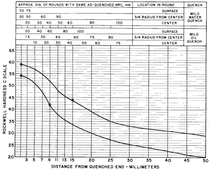
FIG. 17 Limits for Hardenability Band 5140 RH
