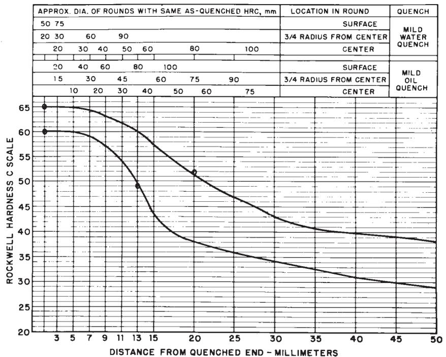
FIG. 18 Limits for Hardenability Band 5160 RH
